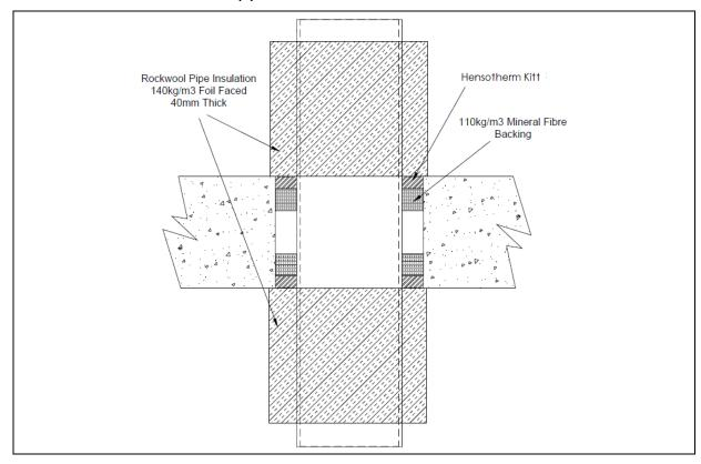
A.3.3.1 Pipes with 40 mm thick/500 mm long, 140 kg/m $^3$  stone wool insulation
