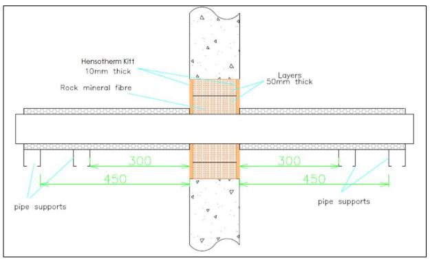
A.1.1.1 Pipes with local interrupted (minimum 500 mm) or continuous 19 mm thick Armacell 'Class O Armaflex' Insulation
