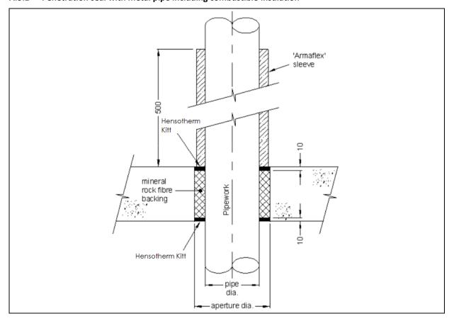
A.3.1.1 Pipes with local interrupted (minimum 500 mm) or continuous interrupted 25 mm thick Armacell 'Class O Armaflex' Insulation
